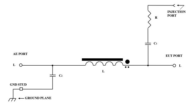
NOTE:  $C_1 = 0.022 \ \mu F (typ.), C_2 = 0.047 \ \mu F (typ.), R = 100 \ \Omega, L = 684 \ \mu H$ Ferrite Beads - as required.
