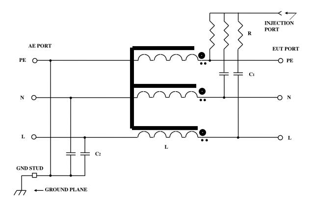
NOTE:  $C_1 = 0.01~\mu F~(typ.),~C_2 = 0.047~\mu F~(typ.),~R = 300~\Omega,~L = 684~\mu H~$  Ferrite Beads - as required.
