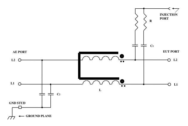
NOTE:  $C_1 = 0.01~\mu F~(typ.),~C_2 = 0.047~\mu F~(typ.),~R = 200~\Omega,~L = 684~\mu H~$  Ferrite Beads - as required.
