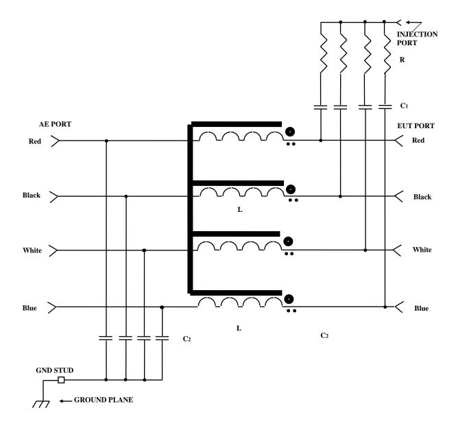
NOTE:  $C_1 = 0.0056 \ \mu F \ (typ.), C_2 = 0.047 \ \mu F \ (typ.), R = 400 \ \Omega, L = 684 \ \mu H$ Ferrite Beads - as required.
