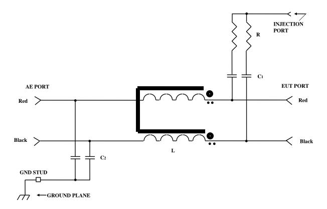
NOTE:  $C_1=0.01~\mu F~(typ.),~C_2=0.047~\mu F~(typ.),~R=200~\Omega,~L=684~\mu H~$  Ferrite Beads - as required.
