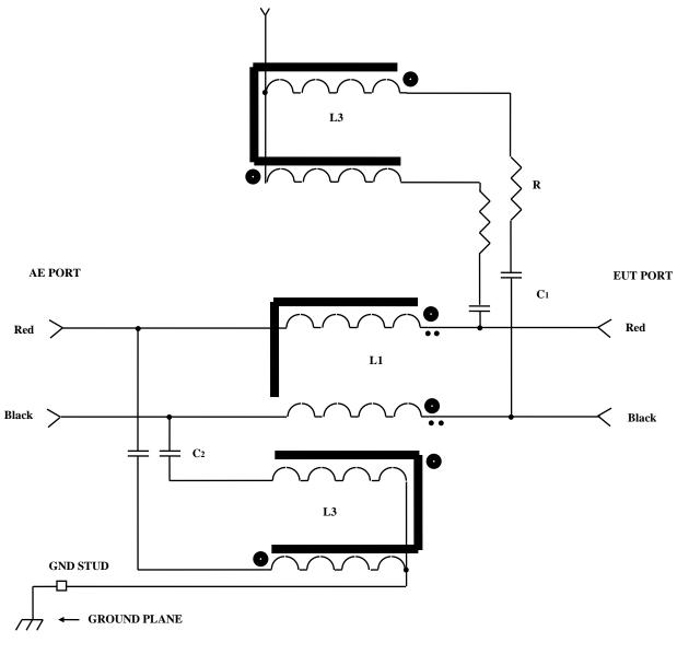
NOTE:  $C1= 0.01 \ \mu F (typ.), C2 = 0.047 \ \mu F (typ.), R = 200 \ \Omega, L1 = 684 \ \mu H, L2 = L3 = 6 \ mH (When C2 and L3 not used, L1 = 280 \ \mu H).$ Ferrite Beads - as required.
