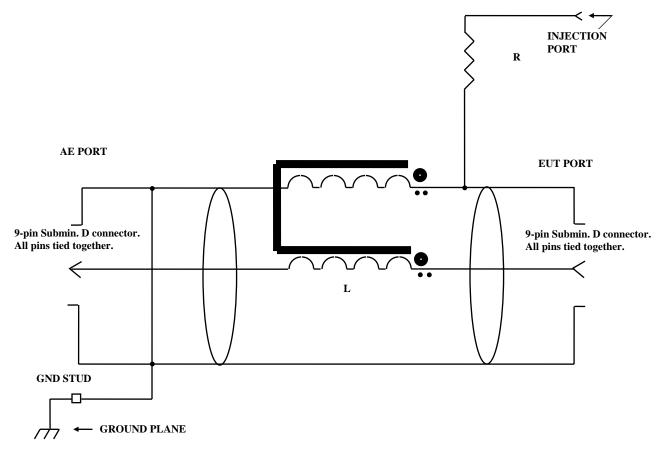
NOTE:  $\begin{array}{ll} R = 100 \ \Omega, \ L \geq 280 \ \mu H \\ Ferrite \ Beads \ - \ as \ required. \end{array}$
