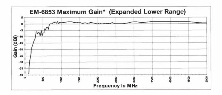
\* Maximum Gain determined from scans at all radiation angles and elevations.
