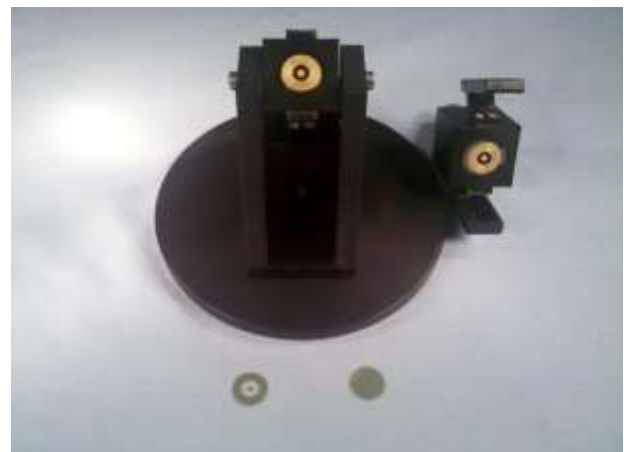
Decoupled Specimen Holder with Gold Reference (left) and Load (right) Inserts in foreground
